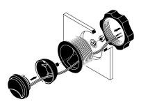
Figure 3. After the Kappa10.1t tweeter is in its cup, hand tighten the nut to flush-mount the assembly on the panel.
